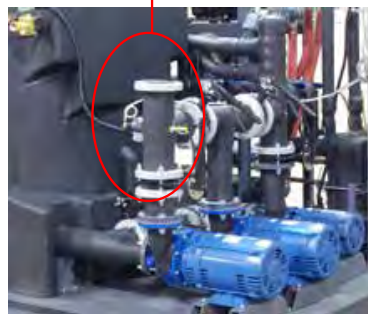
Typical To Process Connection.
