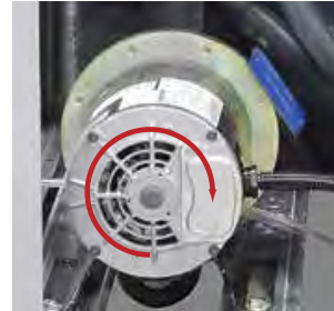
Correct shaft rotation is clockwise.
