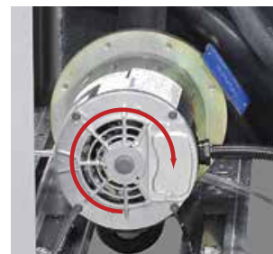
Correct shaft rotation is clockwise.
